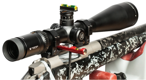
Using bubble levels to square the riflescope to the base.
